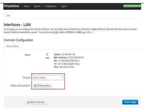
(5) In the static address configuration interface, change the IP address, mask, gateway, broadcast address, and DNS address to the actual planned address of the mine. After editing, click "Save & Apply" in the lower right corner.
