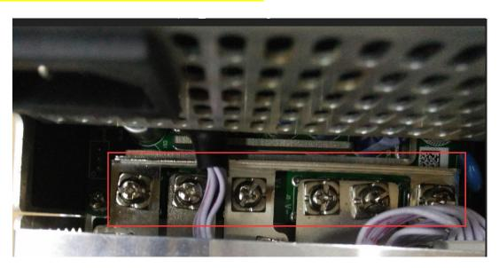
3) Finally, tighten the screws of the four fixed power supplies on the chassis, and the power supply is installed, as shown below:
