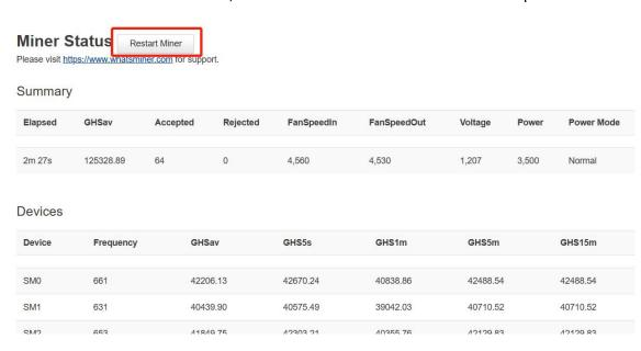
(4) Restart the control board and check whether the configuration modification takes effect. (If you do not choose to restart miner, after the configuration is modified and saved, you can also restart the control board to make the configuration take effect.) In the System interface, click "Reboot".
