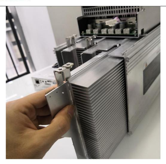
2) After installing the hash board into the miner, first install the adapter board. The socket of the adapter board and the pin of the hash board must be installed in place to avoid other contact related issues, as shown:
