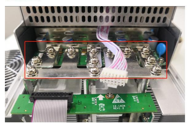
4) After the power bridge is installed, then install control board and the fans, finally the whole hash board installation is done.
