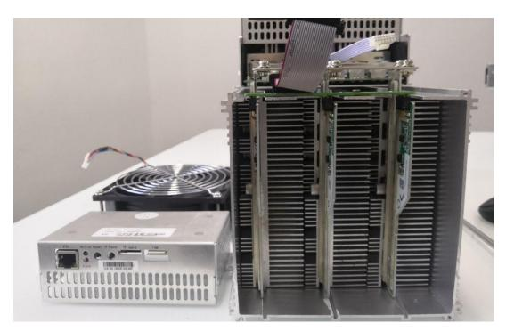
2) Remove the adapter plate and the copper bar fixed to the control panel as shown:
