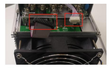
3) Remove the four screws fixed on the bracket and take out the control panel from the bracket as shown:
